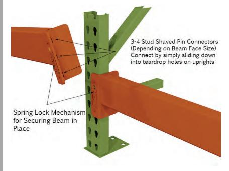
MHE's pallet rack beams come with Shaved Pin connectivity. This makes them compatible with both Teardrop style racking as well as Interlake New Style racking.
